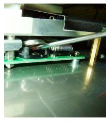
Set the new battery in the battery socket. The positive (+) terminal is upside.
