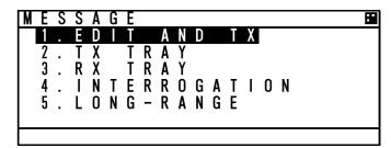
When move the cursor for selecting a desirable item in menu, press ▲ key or ▼ key.
