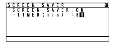
Select "ON", the cursor move to TIMER value. Set the value between 00 and 60 (minutes) with ▲ key or ▼ key and press ENT key.
